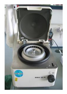
A centrifuge. The centrifuge tubes are placed in the holes around the rim of the central part, which spins fast when the lid is closed.
